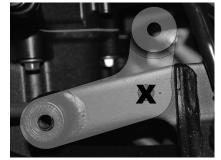
2. Assemble the CFM shift pedal using a threadlocking compound on all bolts except the tip (to be completed in step 6). Bolt the hiem joint to the pedal, placing the spacer between the hiem joint and the pedal (note location for shift pattern below). **IMPORTANT** - Secure all bolts with threadlocking compound.
